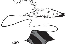
PET bottles are shaved into flakes, then melted into small pellets.
