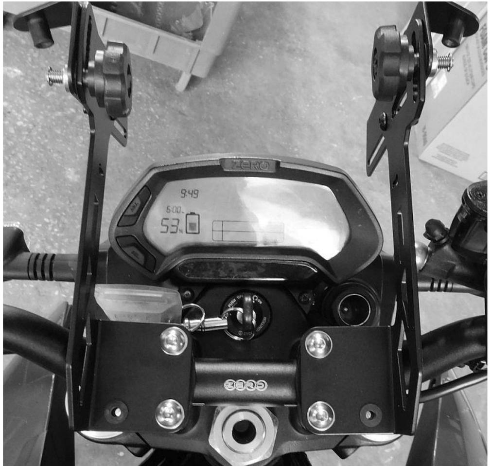
**STEP 1** – Remove the two handlebar clamp bolts ON ONE SIDE ONLY and DO NOT remove the top clamps, only the bolts. (If you remove all four handlebar clamp bolts or your bars will come loose!)
