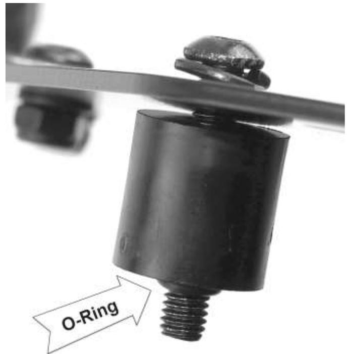
Once all three mounting screws with spacers are in the base plate, set the plate against the front of the bike and screw the bottom two in first (using an M4 Allen wrench), then the center screw. Tighten all three down snugly.
