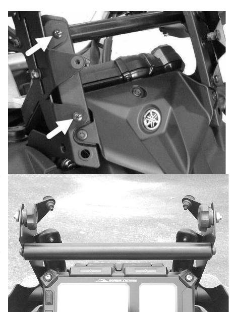
STEP 3: The crossbar you see in these photos gets installed between the two brackets, but there is a pin on one side that must be placed outside of the brackets to keep it from rotating. Please refer to the diagram at right. Before you screw this bar in, go to the next page for the side support step.
