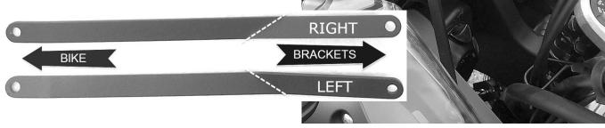
There are two holes down at the sides of the forks for mounting the factory side deflectors (see photo at right). If you have those deflectors then our side supports mount between the deflector and the bike. If you do not have them then insert the M5 well nuts provided (one on each side) into the front hole and attach the side supports to them using the remaining M5 screws with flat washers. Go
