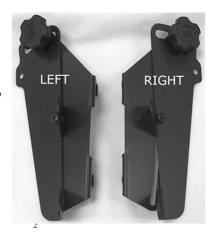
STEP 2: Attach the MadStad brackets to the upper factory mounting holes as shown at right using four of the M5 screws and flat washers provided. Get the screws started and partially snug, but don't fully tighten yet.
