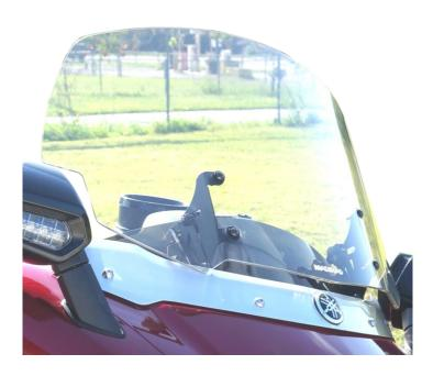
Start with the angle at about the middle of the bracket range, and the top of the shield at about your chin level as you look straight ahead. Then tighten the brackets and go for a ride. Experiment with different positions at different speeds until you find a combination of height and rake angle that eliminates buffeting and gives a smoother ride.
