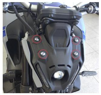
A. Use the M6 x 20 screws from the kit. Be sure the Quik-Release spools are facing outward Repeat the process for the other side of the bike.
