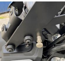
B. Slide the Bracket slots onto the black spools, making sure that the adjustment knobs are facing inward while the Retaining Pins are facing outward. ALSO – be sure the Retaining Pin is locked and secure before riding the motorcycle.
