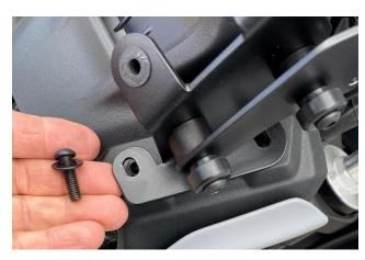
B. The long Support Brace gets attached to the handlebar clamp using (2) M8 X 50 Screw, Aluminum Spacer, and M8 Flat Washer NOTE: Be sure to loosen only one handlebar clamp bolt at a time.
