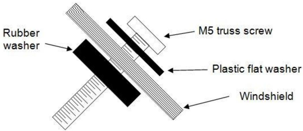
**DO NOT OVERTIGHTEN THE T-SCREWS!** The rubber well nuts cannot be pulled up out of the brackets, even if they are not tight, so tighten only until the well nuts begin to swell up and the shield is snug against the brackets. Over tightening can damage the rubber well nuts.
