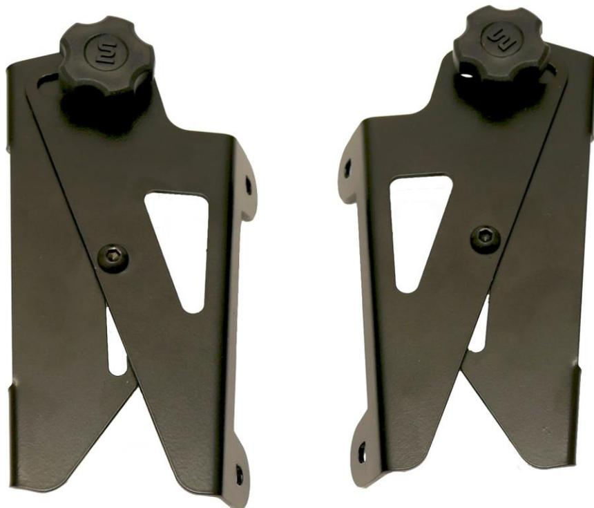
MadStad brackets are designed to bolt to a curved surface like the metal base plate included in this kit. The new windshield attaches to the front of the brackets with quick-removal T-screws. Loosening the two adjustment knobs allow you to change the windshield height and tilt without getting off of the bike, and without any tools.
