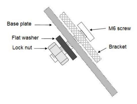
The knobs on the brackets go to the insides (facing each other) with the knob sides up. When both brackets are installed it should look like the diagram below:
