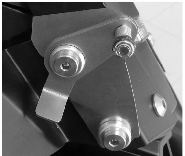
Repeat the process for the left side and lock that bracket into place as well with the locking key.
