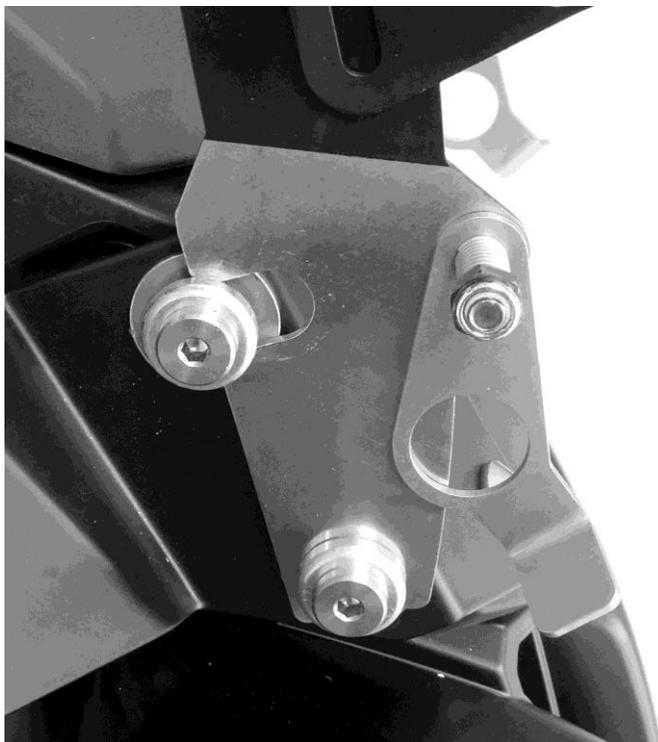
2. Rotate the bracket toward the back of the bike so that the curved slot slides onto the upper spool (see photo at left). Make sure it seats all the way back.
