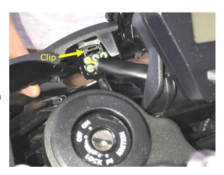
3. Once the wire connector is off, slide the panel down slightly toward the nose of the bike to pop out that bottom tab, then lift the panel off.
