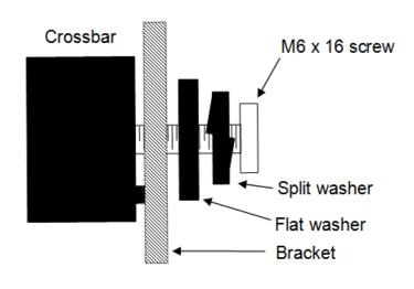
button-head screws with a lock washer and a flat washer and tighten.
