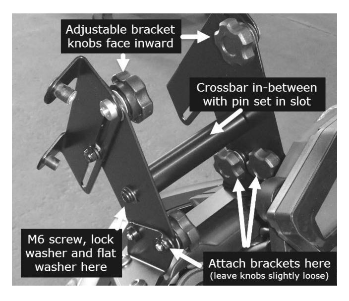
STEP 2: Once both adjustable brackets are in, put the crossbar between them at the crossbar hole in the center of the upright brackets. You will note that there is a hole with a slot, and that the crossbar has a pin sticking out of one end. That pin goes into one of the slots to keep it from rotating. It doesn't matter which side the pin is on, just set the crossbar at the middle screw holes with the pin in one of the slots, then insert the M6
