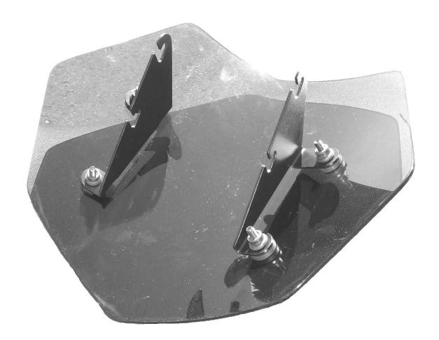
Once the fly screen is assembled, it can be slipped onto the four quick-release knobs on the mounting base. Make sure you slide the fly screen down into the slots, and secure all four knob screws before driving. Please note that the fly screen IS NOT adjustable and is not intended for highway wind protection.
