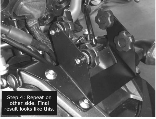
Make sure all six screws are tightened before continuing.
