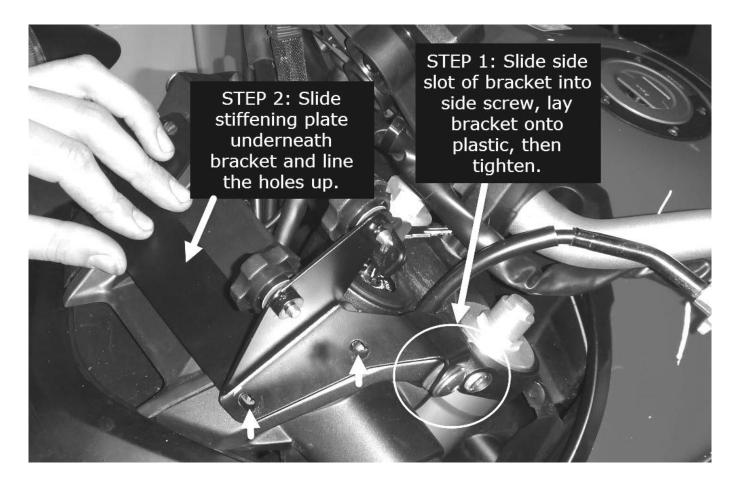
You may want to leave the side screw just slightly loose while you line up the two front holes with the adapter plate and rubber well nuts in the bike plastic. However fully tighten the side screw before fully tightening the front screws because this will help pull the front assembly inward for a better fit.
