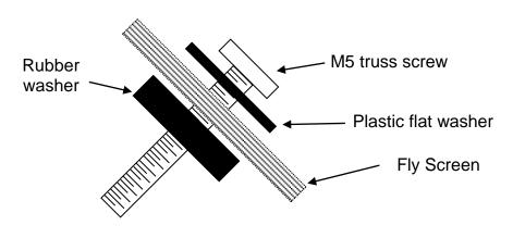
have to assemble the brackets onto the fly screen. Please refer to the hardware diagram above for hardware placement and the photo below for bracket position. Just as with the windshield, do not over-tighten the truss screws; it isn't necessary.
