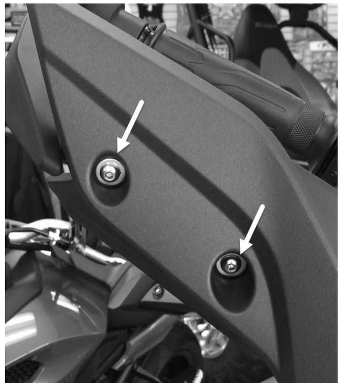
Once the hand guards are apart you will see the two mounting holes in the hand guard frame. You are going to take two black plastic arrow rivets and push them through the inner hand guard (as shown at right) then set that over the frame holes and push the rivets through to snap the two pieces together.
