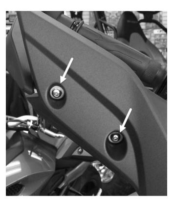
Once the hand guards are apart you will see the two mounting holes in the hand guard frame. You are going to take two black plastic arrow rivets and push them through the inner hand guard (as shown at right) then set that over the frame holes and push the rivets through to snap the two pieces together.
