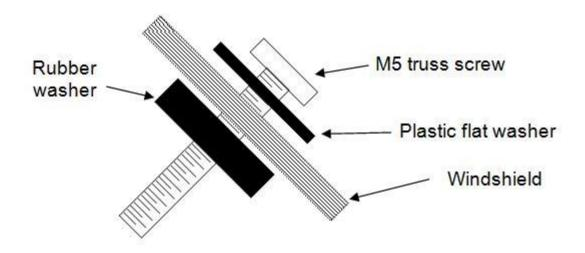
You will probably want to pre-attach these screws and washers to your shield before mounting to the brackets. This will make it easier to get all four screws inserted. The rubber washers on the bottom side will keep the screws from falling out as you handle the windshield.
