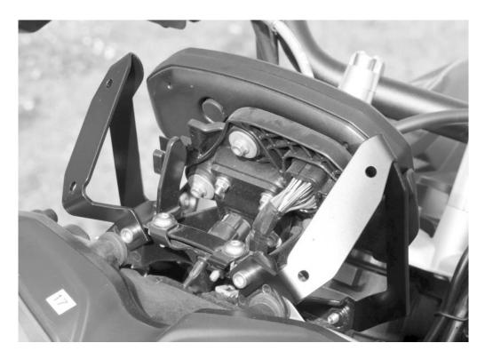
**Step 5**: Line up the aluminum base plate to make sure the four holes in the plate match up to the holes on the two base brackets as shown below. Rotate the base brackets slightly to change their position so their holes line up evenly against the back of the plate, and once they do finish tightening the four base bracket screws. NOTE: The reason you can't just go ahead and attach the plate is because the two front screws will not be accessible once the plate is on.
