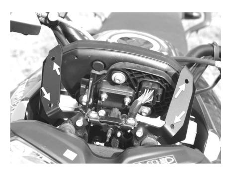
**Step 6**: Attach the plate and adjustable brackets together onto the bases. This means the M6 x 12 button screws go through the brackets, then the plate, then into the base brackets with a washer and lock nut tightened down on the back side of the bases (use M4 Allen and M10 crescent wrench). See photos below.
