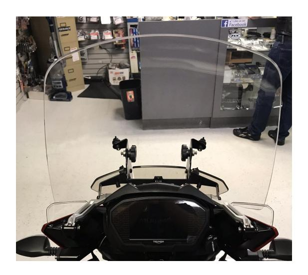
The final installation should look like the photo above. The electric up/down system still works but you probably won't need it. Set the shield height and angle as explained in the next section, with the electric system fully down.
