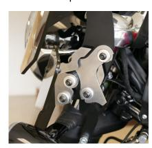
Pull up on the locking tab and rotate between the spools. You may need to push on the spring from the inside.
