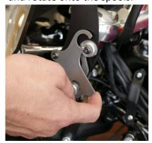
5. Make sure the locking tab is fully pushed down over the two spools.
