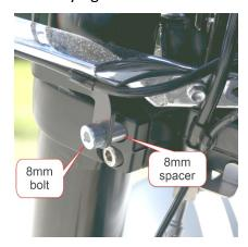
Remove the factory bolt on the top fork clamp. Install bracket as shown then fully tighten both top and bottom.
