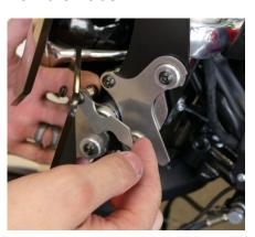
Make sure the locking tab is fully pushed down between the two spools.
