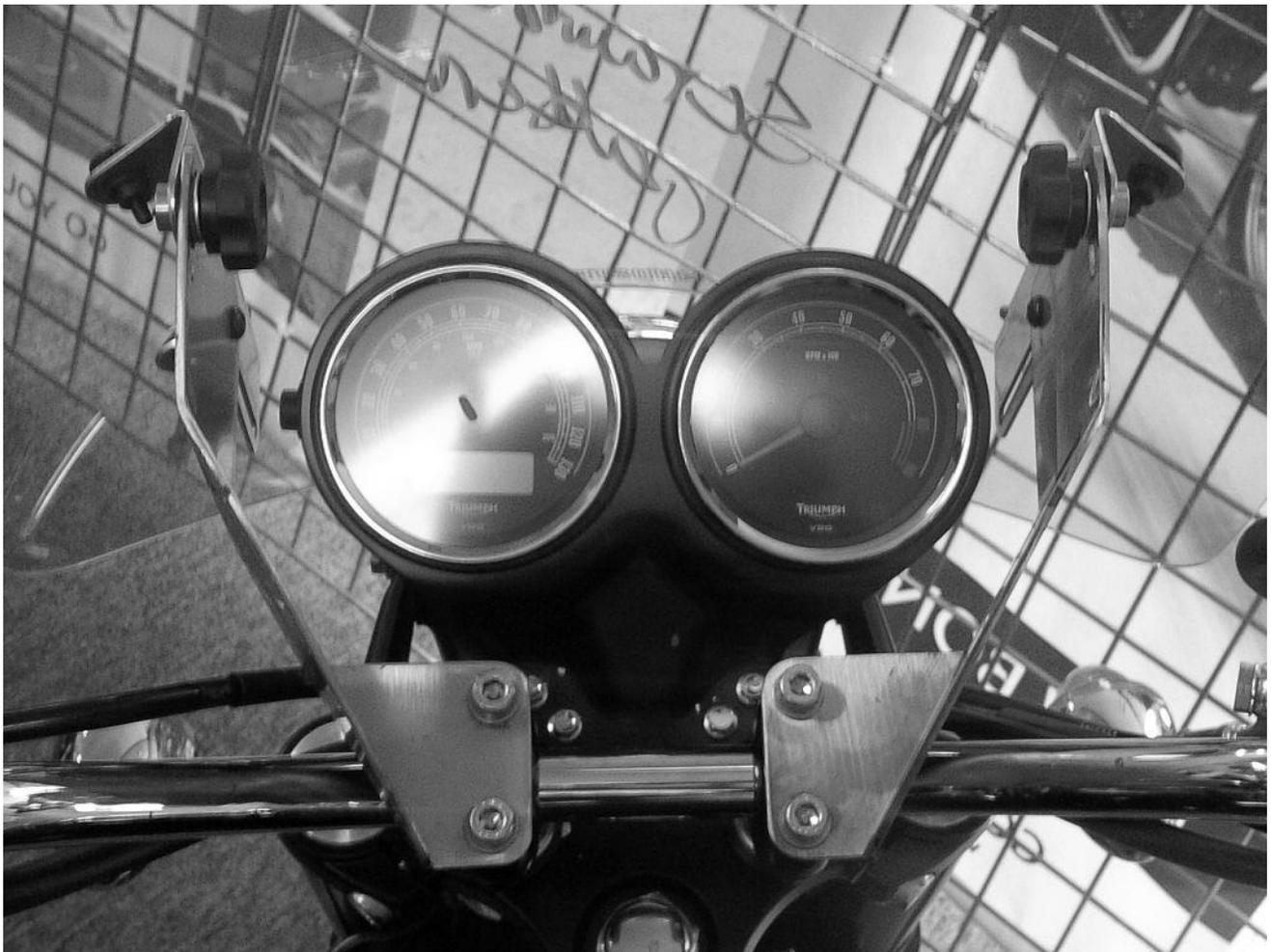
This MadStad system attaches above your handlebar clamps using aluminum spacers and longer bolts. Your handlebars do not need to come loose as you can install these brackets one side at a time.
