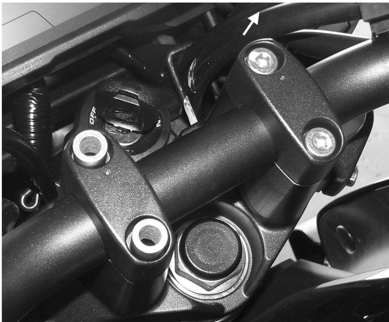
**STEP 3** – Set two of the M8 bolts with flat washers through one of the two MadStad brackets. On the other side put another flat washer and then a spacer on each bolt. This setup will go in through the handlebar clamp and bolt down. The complete picture of how the bolts, washers, spacers and clamp go together is shown below:
