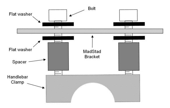
**STEP 4** – Take this the bracket-and-hardware assembly and bolt it down.
