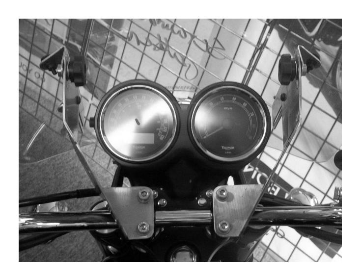
This MadStad system attaches above your handlebar clamps using aluminum spacers and longer bolts. Your handlebars do not need to come loose as you can install these brackets one side at a time.
