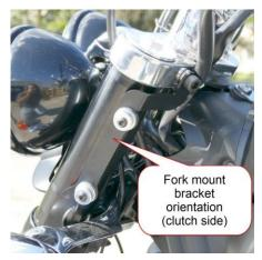
Remove the factory top bolt on the bottom fork clamp. Install bracket as shown below but do not fully tighten.
