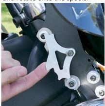
5. Make sure the locking tab is fully pushed down over the two spools.
