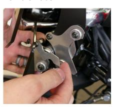
Make sure the locking tab is fully pushed down between the two spools.
