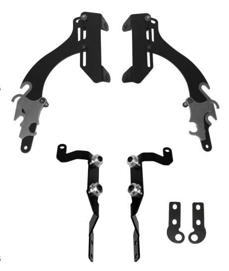
The image at right shows the fork mount brackets and the bottom tabs. The brackets attach to the top fork clamp bolt, the small tabs attach to the bottom fork clamp bolt and then they connect together to form a complete bracket. They are in two parts because you do not want to loosen both fork clamp bolts at the same time, your fork tube could slip out of position. Install these in the order shown below.
