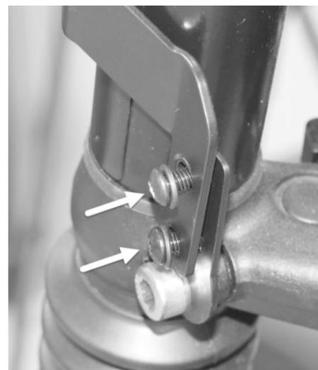
**Step 4:** Once both fork brackets are bolted to the top of the forks and lined up with and overlapping with the bottom tabs, screw the brackets to the bottom tabs using the M6 screws with flat washers and lock nuts on the back side.
