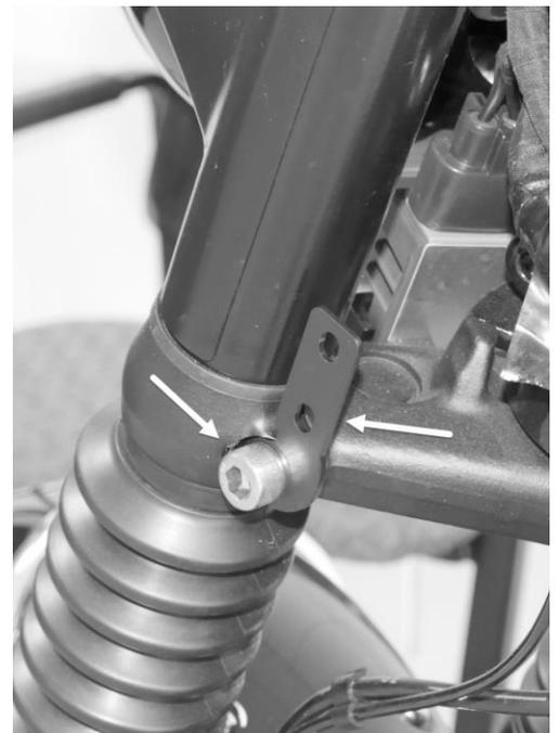
**Step 2:** Before installing the main fork mount bracket, place a rubber bumper at the back of each or the two screws as shown in the photo below. When installed the tips of these screws are right up against the fork tube so we don't want them scratching the tube. Extra adhesive bumpers have been provided if necessary.
