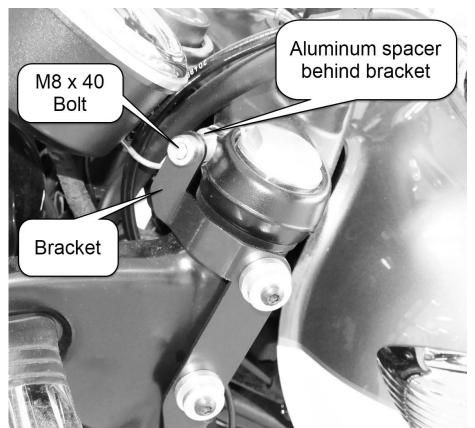
d. Tighten fork clamp securely. As you do this, check the alignment of the bracket with the tab installed in step #1. They should overlap. e. Run the M6x16 screws into the overlapping holes to keep aligned as you go to tighten the top fork bolt.
