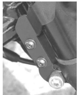
The quick-release windshield brackets will snap onto the aluminum spools on these brackets, and you will do that first before attaching the shield to the brackets.
