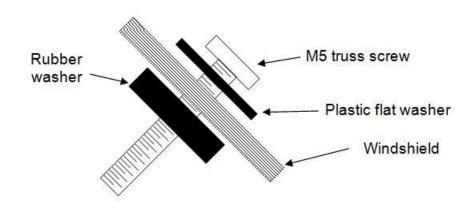
**b.** Set up all four screws in the four windshield holes. **c.** Bring the shield over the brackets and set the screws into the rubber well nuts. Screw them in until the rubber of the well nut swells and makes a secure connection. Do this for all four screws until the windshield is secured to the brackets.
