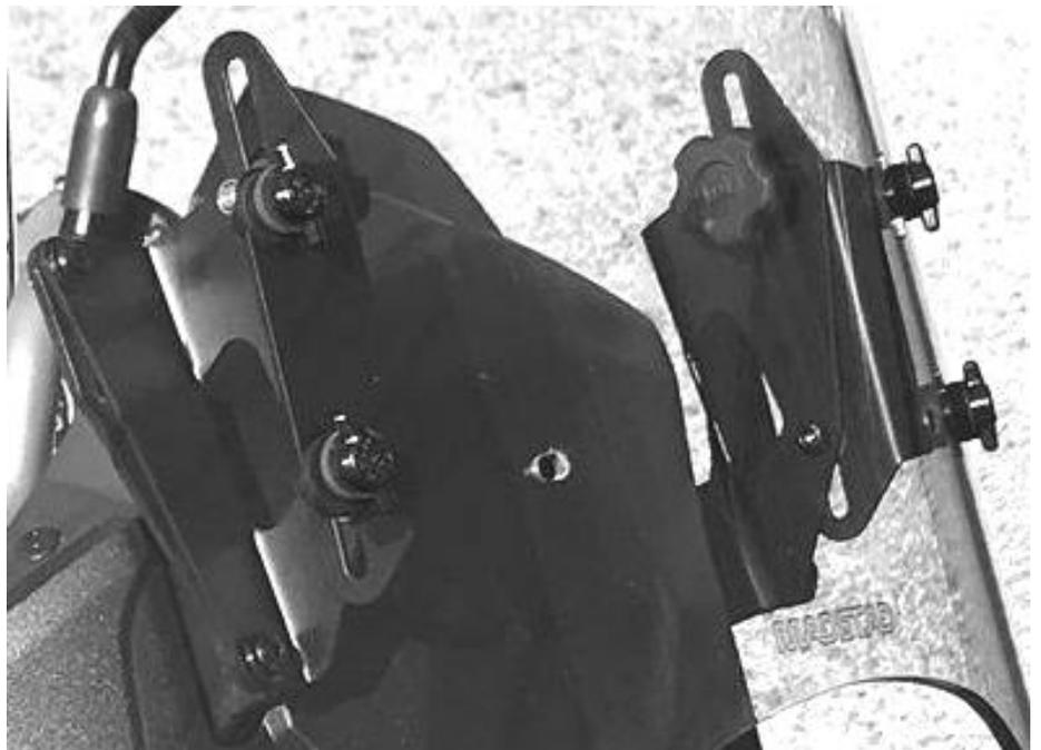
The MadStad adjustable windshield brackets are designed to bolt to the factory windshield brackets (metal plates). The MadStad windshield then attaches to the front of the brackets with quick-removal T-screws. Loosening two adjustment knobs on the brackets allows you to change the windshield height and tilt without getting off of the bike and without any tools.
