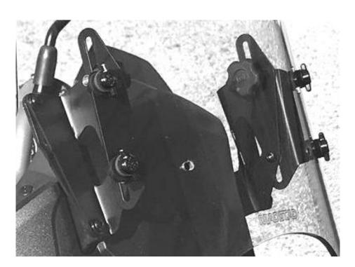
The MadStad adjustable windshield brackets are designed to bolt to the factory windshield brackets (metal plates). The MadStad windshield then attaches to the front of the brackets with quick-removal T-screws. Loosening two adjustment knobs on the brackets allows you to change the windshield height and tilt without getting off of the bike and without any tools.
