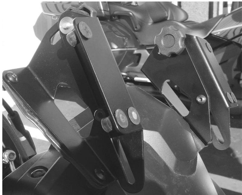
These MadStad adjustable windshield brackets are designed to bolt to the factory windshield holes. The MadStad windshield then attaches to the front of the brackets with quick-removal T-screws. Loosening two adjustment knobs on the brackets allows you to change the windshield height and tilt without getting off of the bike, and without any tools, and without needing to use the factory height adjusters.
