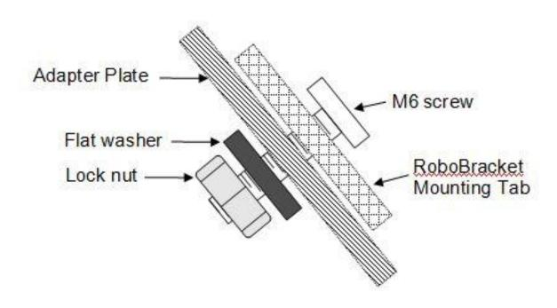
The knobs on the brackets go to the insides (facing each other) with the knob sides up. When both brackets are installed it should look like the diagram below:
