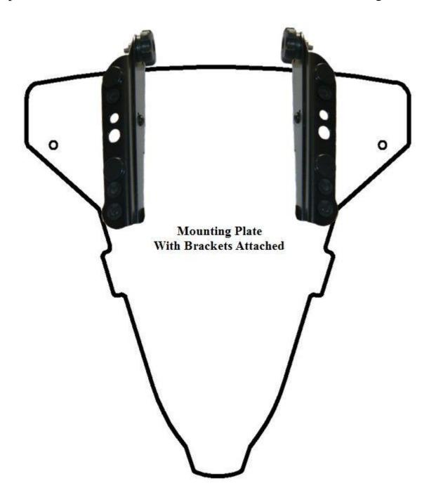
The adapter plate then slides into the fairing in place of the stock shield. You may have to wiggle it around a bit to get all the holes lined up, then screw it in with the original factory windshield screws and washers.
