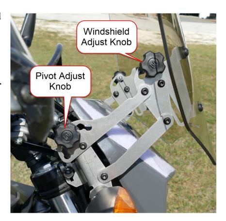
Once both brackets are in the same position then the windshield can be installed.
