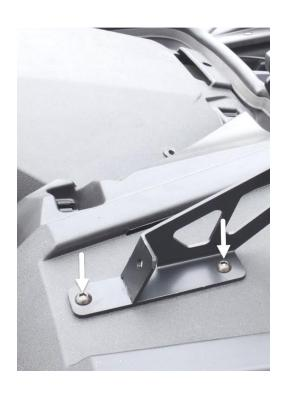
**STEP 6**: Install the MadStad bases. There is a left and right acrylic base which our adjustable brackets bolt to. They are shown below as if you are looking at them from the front of the car. You can't install them incorrectly; they will only fit one way!
