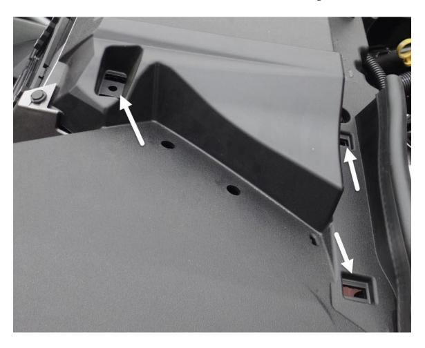
**STEP 4**: Insert the provided M6 well nuts into the round holes you just exposed.
