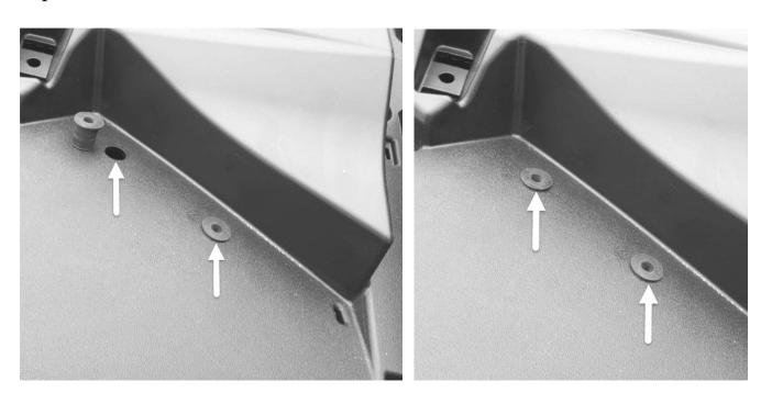
**STEP 5**: Remove the radio. First you need to remove the four screws at the corners of the bezel (cover plate). You will need a very small 2.5mm Allen wrench.
