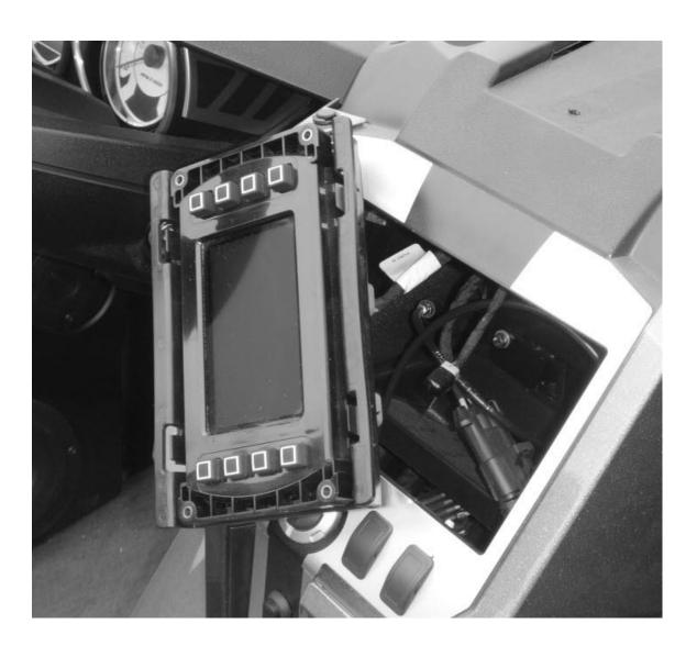
**STEP 5**: Remove the center support post. If you don't have one then just pull out the two plastic plugs that are in the center of the dash. Otherwise, remove the two screws as shown below, and before the second one falls out put your hand in under the dash and grab the aluminum mounting plate that was holding these two screws in (shown below). You won't need these parts.
