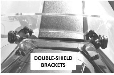
STEP 6: Install the windshield. Before you set the windshield onto the brackets, pre-install the outer four mounting screws and their washers as in the diagram at right. One rubber washer sits against the front of the windshield with the
