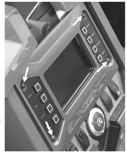
Once the radio cover plate is off, extract the radio by pushing the four locking tabs inward to unsnap it from the dashboard housing. When the unit comes loose, gently pull it out and let it hang off to the side, or pull the plugs off of the back and remove it altogether. However you don't necessarily need to do that; you just need to be able to get your hand in to reach up under the center of the dashboard.
