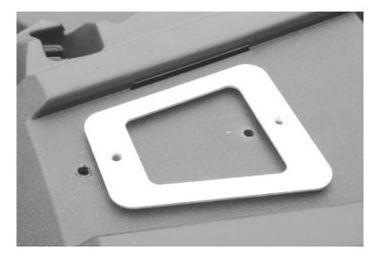
**STEP 6**: Install the MadStad center post. We have provided a much stronger and stiffer brace plate (see below) and this goes in up underneath the two center dash holes. The rubber bumpers must be facing up. Hold this plate in place underneath the dash and line up the holes. Then set our center post on top and screw it in with the M6 x 20mm screws provided and a lock washer under each screw head.
