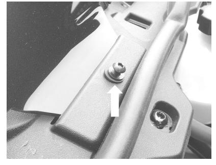
Line up the other three base holes with their corresponding well nuts, insert an M6 x 25 screw with plastic washer through these holes then snug all four screws up. There is no need to tighten hard; simply tighten until they are good and snug.
