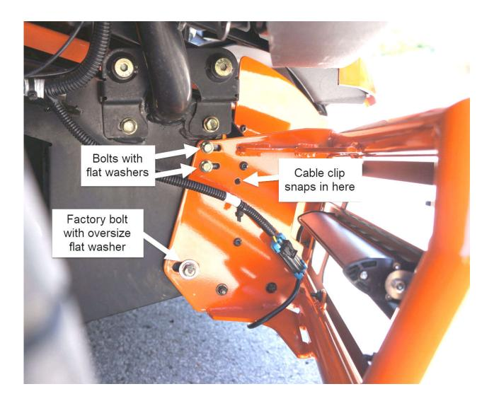
Once the bumper is securely on the frame, make final adjustments to the Center Assembly so that it is evenly lined up with the hood, and with minimal gap between the center and hood. Make sure the hood is fully closed and latched before you make final adjustments. Tighten all 8 of the screws and nuts that were left loose once everything is lined up.
