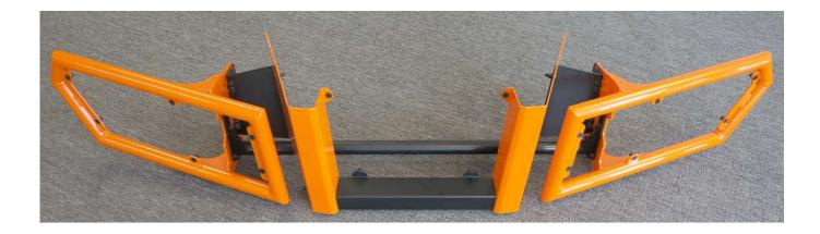
**Step 5 – Hardware D:** The bumper assembly can now be bolted to the Slingshot frame, back onto the same holes as the factory wing (see image below). Use the two bolts we provide for the upper two holes, and use the original factory bolt for the bottom but put our oversize flat washer on it first. Don't fully tighten these bolts until you check out the bumper alignment from the front. Adjust as necessary then tighten all six of these bolts.
