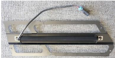
Step 7 – Hardware F: The bumper inserts and center grille can now be mounted into the rubber well nuts on the bumpers and center assembly. A plastic flat washer goes under the head of each screw, and make sure you do not over-tighten these screws or you could damage the well nuts! The rubber well nuts swell up and will hold these inserts in place, so you just need to make sure the screws are snug, not cranked down hard.
