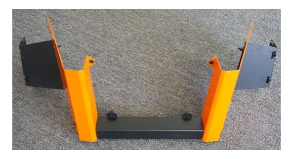
Step 3 – Hardware C: The left and right Bumpers get connected together by the Crossbar as shown below. Screws with flat washers under the head go through the crossbar into the bumpers, then put another flat washer and nylock nut on the inside of the bumper. Snug all six up but don't fully tighten. First make sure both bumpers are even with each other on the crossbar. Once they are, tighten all six screws and nuts fully. This now becomes the **Bumper Assembly** (see below).
