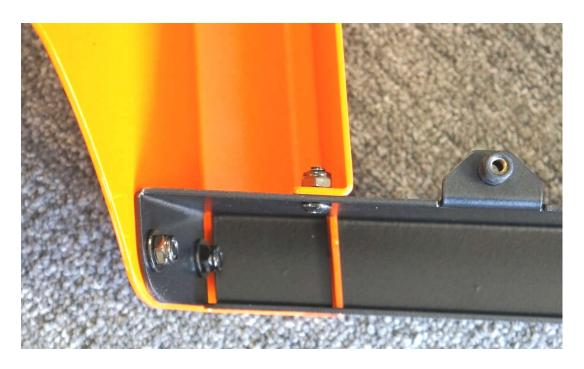
Step 2 – Hardware B: Attach the center mounting plates as shown here. DO NOT FULLY TIGHTEN THESE SCREWS! Each of these plates needs to be a little loose so that you can adjust the position once the entire bumper is on the vehicle.
