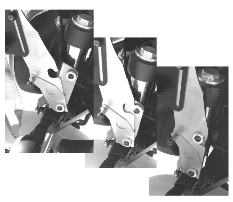
To lock the brackets in, pivot the locking tab up and onto the upper button, and allow it to snap completely over (see photos below). You might have to wiggle the buttons or bracket around a bit but make sure the locking tab snaps <u>fully</u> down around the button.
