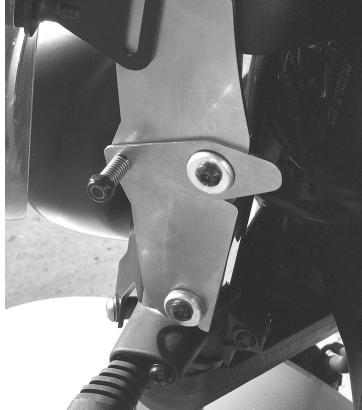
Once the brackets are snapped onto the buttons it is time to tighten those buttons down using a 4 mm Allen wrench and a 10 mm openend or box-end wrench (see photo at right). Make sure you tighten both the upper and lower buttons. Repeat this bracket installation process on the other side.
