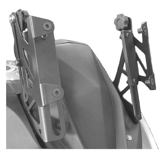
MadStad adjustable windshield brackets are designed to bolt to the same factory slotted brackets that the factory shield slides up and down on. However our brackets have their own height adjustment *and* angle adjustment so they will be bolted down into place. You will then be able to change the windshield height and angle without getting off of the bike, and without any tools. The factory windshield is not adaptable for use with these brackets.
