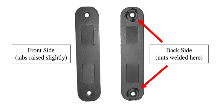
The knobs on the brackets go to the insides (facing each other) and up at the top (as seen below). When both brackets are installed they should look like the image on Page 1. You will want to have the four M6 x 20mm screws ready with a split-ring lock washer on each, as well as an M4 Allen wrench. You may need to loosen the bracket knob a turn or two so you can slide the bracket open to a position where the screw holes are easily accessible.
