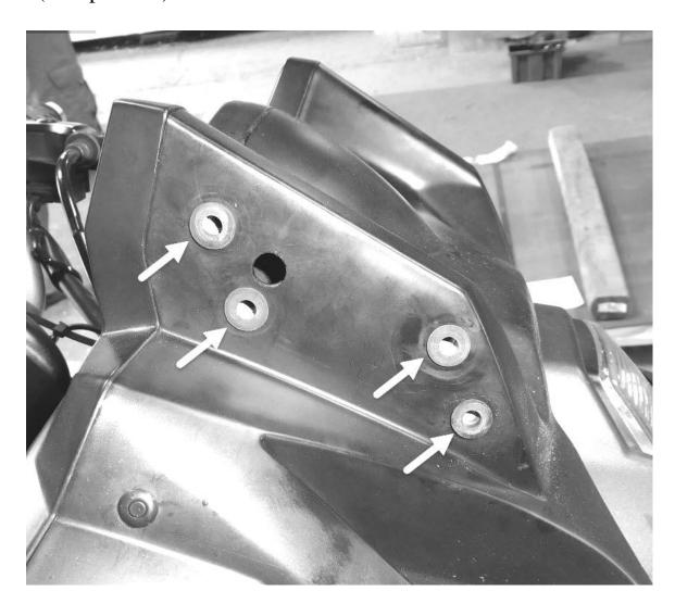
**STEP 2:** Attach the MadStad brackets to the well nuts using the Phillips screws and flat washers provided. The black adjustment knob should be up and facing each other. Use the photo at right for reference.
