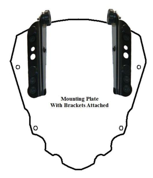
The adapter plate then **slides into the fairing** in place of the stock shield. You may have to tilt it a bit to get the rubber well nuts (which are in the bottom two holes) over the instrument cluster but it will slide in. Then install the bottom two factory screws into the bottom two well nuts and tighten. You will install the top two screws in the next step.
