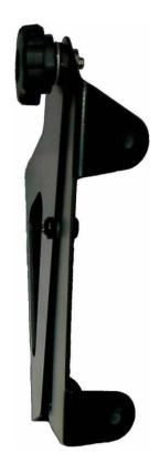
MadStad adjustable brackets are designed to bolt to a curved surface like the mounting plate included in this kit. The new windshield attaches to the top of the brackets with the M5 Phillips truss screws, flat plastic washers, and soft rubber washers. Loosening the two adjustment knobs allows you to change the windshield height and tilt without getting off of the bike, and without any tools.
