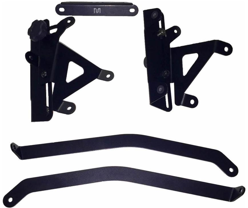
These MadStad adjustable brackets are designed to bolt to the factory windshield holes. The MadStad windshield then attaches to the front of the brackets with quick-removal T-screws. Loosening two adjustment knobs on the brackets allows you to change the windshield height and tilt without getting off of the bike, and without any tools, and without needing to use the factory height adjusters.
