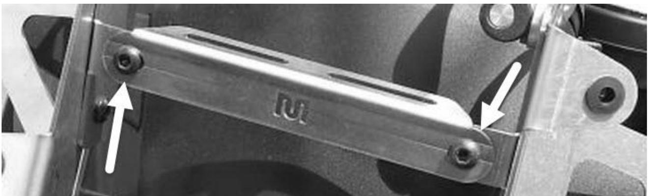
**REAR BRACES** – There are two long braces that go from the rear tab on the MadStad brackets down inside the fairing to factory mounting points which are to the left and right of the forks. If you look down where your forks are you will see two screws that run straight down through the fairing (see photo at right). Remove the screw that is toward the front of the bike (as shown by the arrow). Leave the round spacer/washer behind, our brace will bolt right over it.
