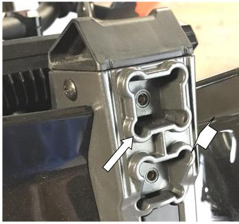
The MadStad bracket assembly gets placed onto the factory shield mount with the two short screws that are poking out of the back of the plate placed into the two semi-circular recesses as seen at left. This will orient the two mounting screw holes directly over the factory threaded holes. Insert the top screw first and tighten down, then insert and tighten the bottom screw. The final result should look like the image below.
