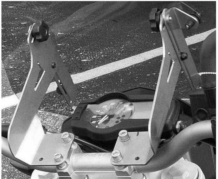
This MadStad system attaches above your handlebar clamps using aluminum spacers and longer bolts. Your handlebars do not need to come loose as you can install these brackets one side at a time.
