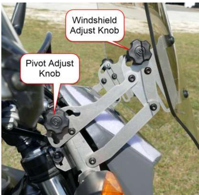
into one of the seven holes on the pivot bracket. We recommend you start out with both brackets pivoted fully up and back for windshield installation. Also make sure the windshield adjustment mechanism (upper knobs) is the same on both sides, otherwise the windshield won't line up to the brackets. Loosening the knobs just one turn will free up the height adjustment. To change the windshield angle, loosen about 3-4 turns.
