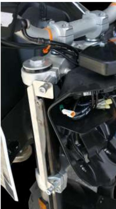
**STEP 5** – Install our fork bracket as shown in the photo at left. The long bolt goes through the top hole of our bracket with the long spacer between the bracket and the bike. The shorter bolt goes through the bottom hole of our bracket with the shorter spacer between the bracket and the bike.
