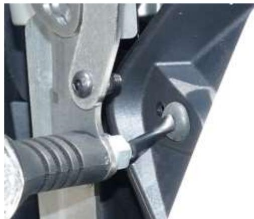
**STEP 9** – Set the grommets into the sides of the head light housing. You may want to use a small flat-blade screwdriver or similar tool to help you push the grommet into the hole.
