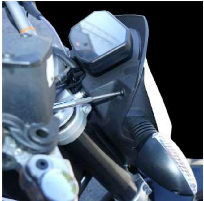
**STEP 2** – Disconnect the wires to the turn signals and headlight. You will need a small pointy tool or small flat-blade screwdriver to push on the connectors and unlatch them. Make note of which turn signal goes to which wire so that you can match them back up when putting it back together.
