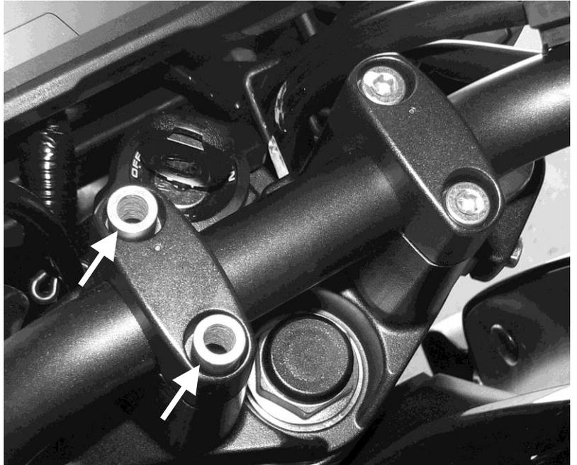
**STEP 2** – Set two of the aluminum spacers provided in your kit into the two holes in the now-open top clamp, as seen in the photo above. Put one M8 flat washer on top of each spacer. To keep it from slipping off, put a dab of Vaseline or similar thick grease on top of the spacer so that the flat washer will stick to it and not slide off.
