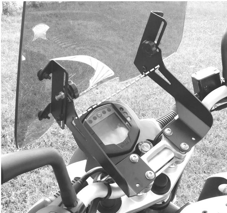
**STEP 5: Crossbar** – The solid aluminum crossbar mounts between the two adjustable brackets as shown at left. One side of the crossbar has a protruding pin which must sit in the slot on either bracket, to prevent the crossbar from rotating. Slide the crossbar between the brackets, align the center hole with the keyhole slot in the bracket as shown below, then fasten as shown below. The finished assembly should look like the photo at
