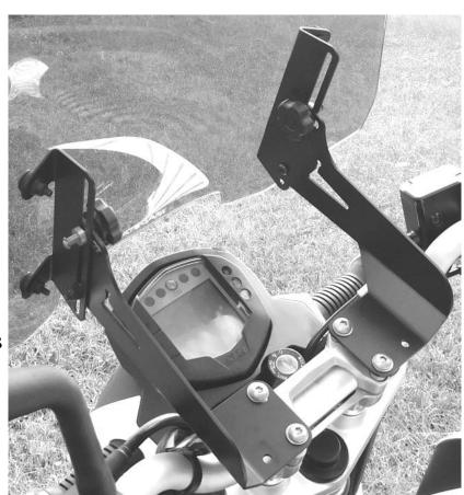
This MadStad system attaches above your handlebar clamps using aluminum spacers and longer bolts. Your handlebars do not need to come loose as you can install these brackets one side at a time.
