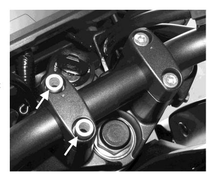
**STEP 2** – Set two of the aluminum spacers provided in your kit into the two holes in the now-open top clamp, as seen in the photo above. Put one M8 flat washer on top of each spacer. To keep it from slipping off, put a dab of Vaseline
