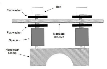
**STEP 3** – Insert the bracket with the new M8 bolts and washers provided right through the aluminum spacers and into the mounting holes of the bottom bar bracket. Run the bolts in with your fingers to get them started then bolt them down so the final result looks like the photo below. **NOTE**: Tighten the front bolt completely first, then tighten the back bolt to factory specifications.
