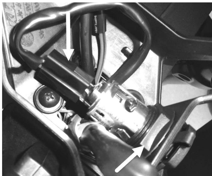
**STEP 3:** – Remove the cigarette lighter socket by pulling the plug off of the end, then unscrewing the plastic nut. Pull it completely out of the mounting hole.
