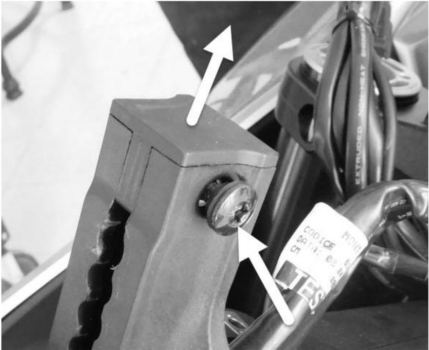
**STEP 6:** – Feed the wiring harnesses through the bottom of our mounting base and set it onto the mounting platform of the bike. Then feed through the factory instrument panel bracket and set it on top of our base plate. Fasten down through both using the MadStad Phillips screws provided. Then re-attach the instrument panel.
