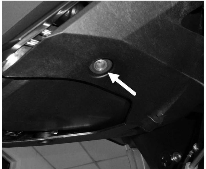
**STEP 4:** – There are four screws behind the headlight housing, two above and two below as shown above. Remove them and hold onto them. This allows you to pivot the small fly screen and headlamp assembly forward, which you will need to do in a minute to remove the factory windshield bracket.
