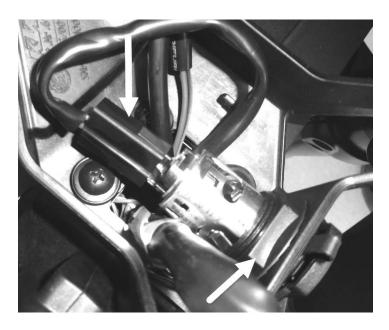
STEP 4: – Remove the four factory screws holding the instrument panel base to the bike. Pull this plastic base off carefully over the wiring harnesses. You WILL NOT be reusing these screws, but save them somewhere with the other bike parts being removed.
