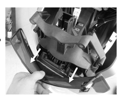
STEP 5: – There is a side screw at the top of the windshield adjustment. Remove that screw and pull the cap up off of the stem. You should then be able to tilt the flyscreen forward a bit and slide the factory windshield bracket up and out of the stem. After that, replace the cap, cap screw and the four headlight housing screws you removed in Step 4.
