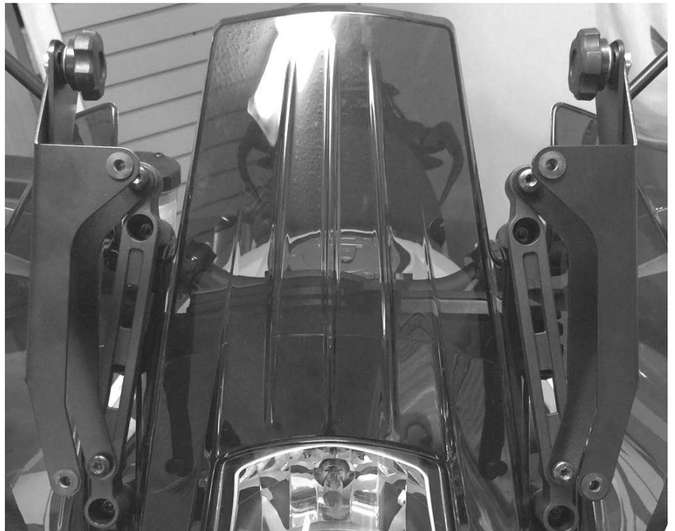
These MadStad adjustable windshield brackets are designed to bolt to the factory windshield mounting points and the factory shield (or any other aftermarket shield made for the 1290 SA) attaches to the front of our brackets.
