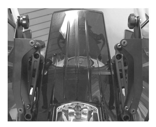
These MadStad adjustable windshield brackets are designed to bolt to the factory windshield mounting points and the factory shield (or any other aftermarket shield made for the 1290 SA) attaches to the front of our brackets.
