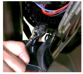
B. There are also two screws that have to be removed right above the headlight, on the headlight shroud.
