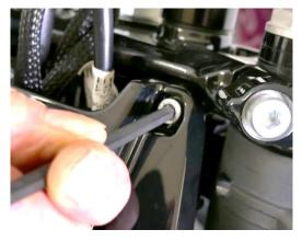
C. The Headlight Shroud sits on two welded-in screws off of the fork clamp. When removing the shroud and headlight, lift slightly up and then pull away.
