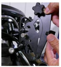
The MadStad Quick-Release Brackets slide onto the black spools that are on the base bracket. They have a spring pin locking mechanism. Pulling out the pin head then rotate it counter-clockwise to lock the pin into the open position. Turning clockwise will release the pin to go forward and lock into place. Be sure the adjustment knobs are facing outward and that the locking pin is through the hole in the bracket.
