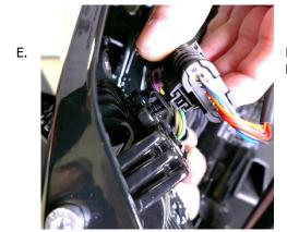
Disconnect the electrical connector going into the back of the headlight as seen below, then remove the headlight.
