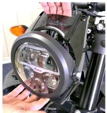
D. There are two wiring clusters – one for the headlight and the other for components. Both are attached to the back of the headlight by a plastic retainer clip. They can be simply pulled out, away from the headlight.
