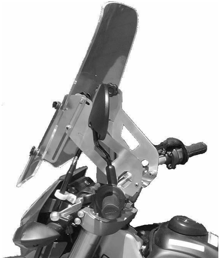
You will not need to loosen the handlebars to perform the installation so your bars will stay in position. You will also be able to remove the MadStad adjustable brackets and shield completely and easily should you decide to go off-roading.
