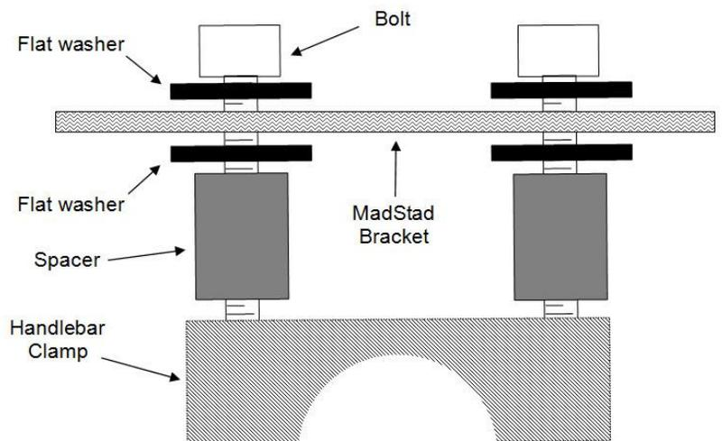
Slide the bar clamp bracket under the crossbar then insert both bolts back into the top clamp, making sure there is a flat washer between our bracket and the factory top clamp. Tighten the front bolt completely first, then tighten the back bolt to factory specifications.
