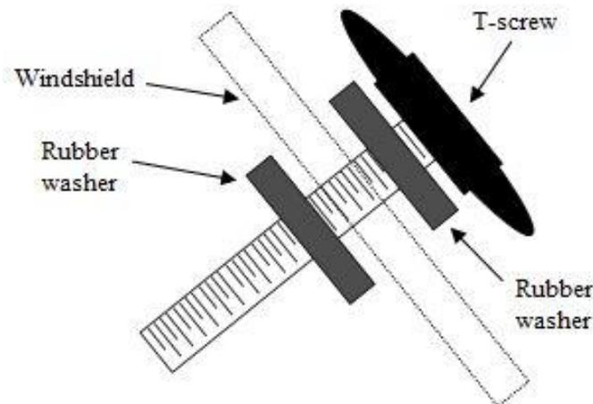
**DO NOT OVERTIGHTEN THE T-SCREWS!** The rubber well nuts cannot be pulled up out of the brackets, even if they are not tight, so tighten only until the well nuts begin to swell up and the shield is snug against the brackets. Over tightening can damage the rubber well nuts.
