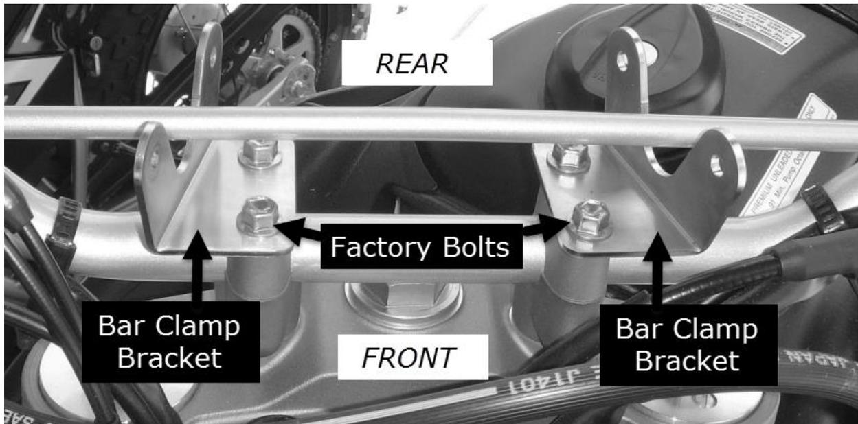
**STEP 2** – Run two M8 bolts (provided) through the Bar Clamp Bracket for that side (see photo above) and add a flat washer under each bolt head. (See hardware diagram below). Use aluminum spacers between the bar clamps and brackets to raise the brackets up off of the bar clamp curvature. Use the extra flat washers on top of each spacer if you feel you need the extra clearance over the bar clamp.
