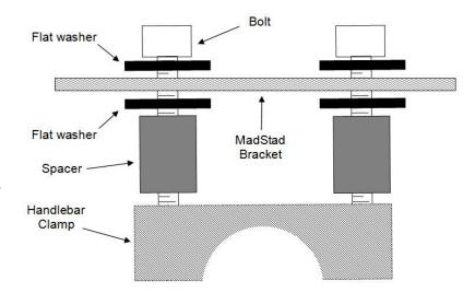
factory top clamp. Tighten the front bolt completely <u>first</u>, then tighten the back bolt to factory specifications.
