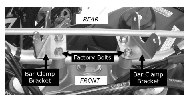
**STEP 2** – Run two M8 bolts (provided) through the Bar Clamp Bracket for that side (see photo above) and add a flat washer under each bolt head. (See hardware diagram below). Use aluminum spacers between the bar clamps and brackets to
