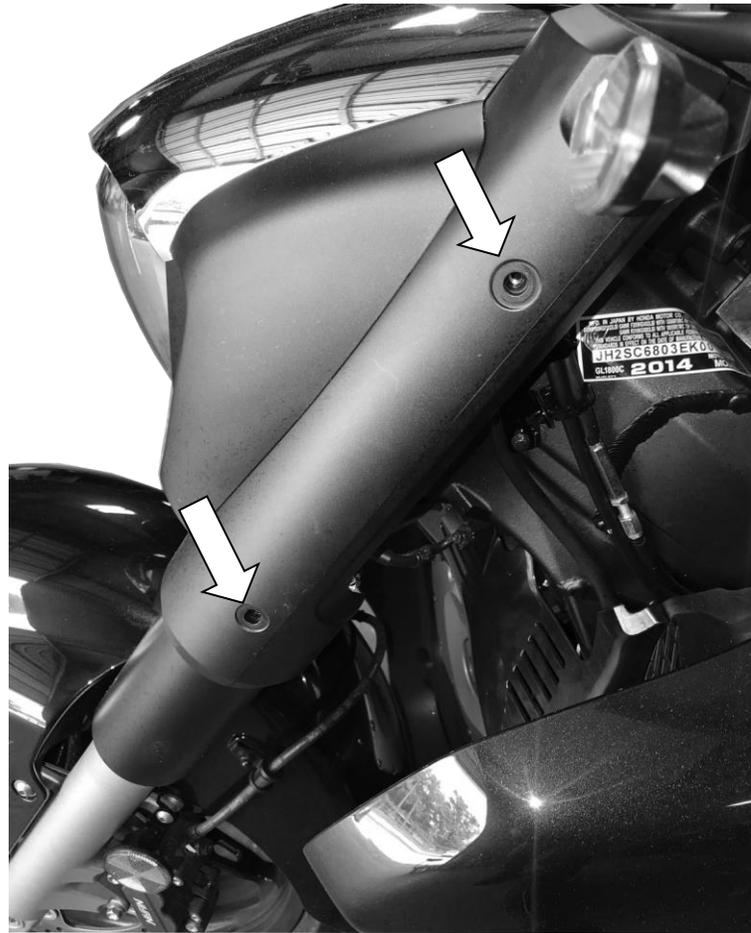
The wide aluminum spacer will slip over the sleeve spacer. Insert the screw and the sleeve spacer goes in through the plastic fork cover, and the aluminum spacer will sit between the fork cover and our bracket. Attach our bracket in this manner. The black knobs on the brackets must face in toward each other and the notch will slide over the turn signal stem. See the photo on the next page for how it should look when installed.
