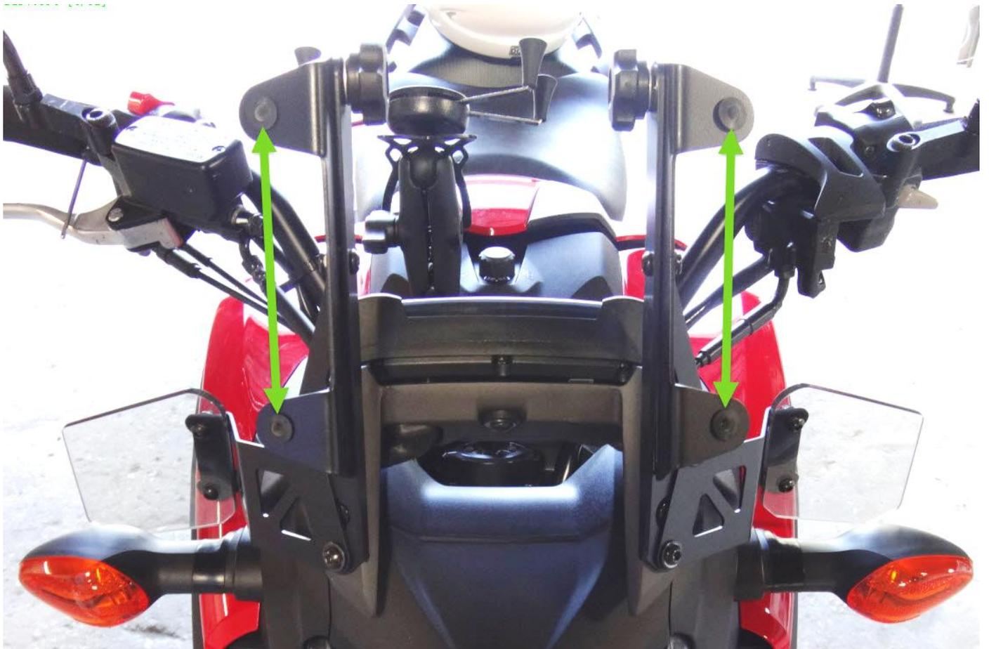
The windshield attaches to the brackets with Phillips truss screws, plastic flat washers and rubber washers as shown below. Pre-install all four screws and washers into the windshield before attaching onto the brackets. Nudge the screws into the well nuts then screw them in until they are snug, which means the screw tip has gone slightly past the back of the well nut. **DO NOT OVERTIGHTEN THE TRUSS SCREWS!** Over-tightening can damage the rubber well nuts.
